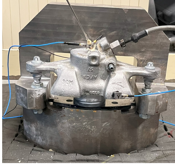
Figure 5: Piston/backplate contact test bench
